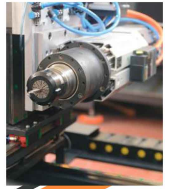
4. Unit Spindle Milling Motor 4. Ünite 9kW HSK F63 HSD Spindle Motor
